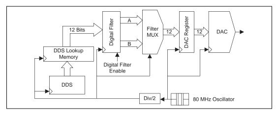
Figure 2-2. Waveform Data Path Block Diagram
